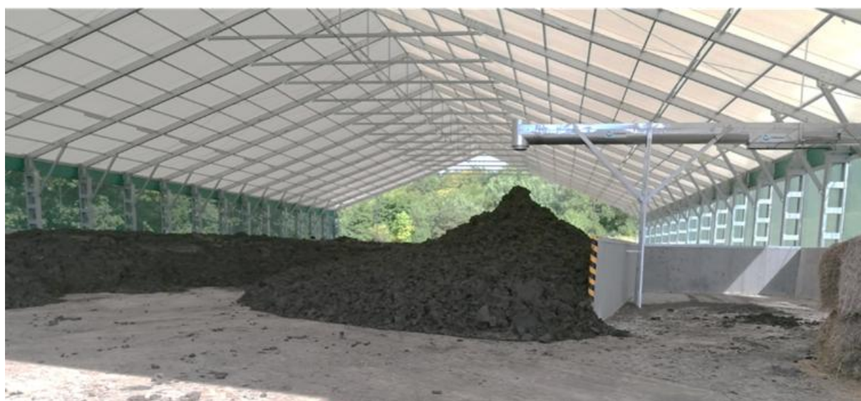
Figure b.30. Final product of sediment treatment in the storage shed (source: Kartuzy WWTP)
