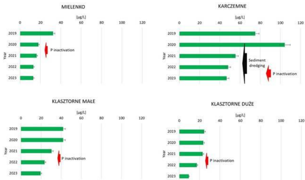
Figure b.7. Changes in average annual concentrations of chlorophyll a in Kartuzy Lakes during restoration treatments
