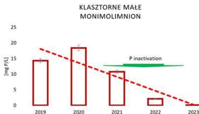
Figure b.4. Changes in average annual concentrations of total phosphorus in monimolimnion of Klasztorne Małe Lake during and after restoration treatments
